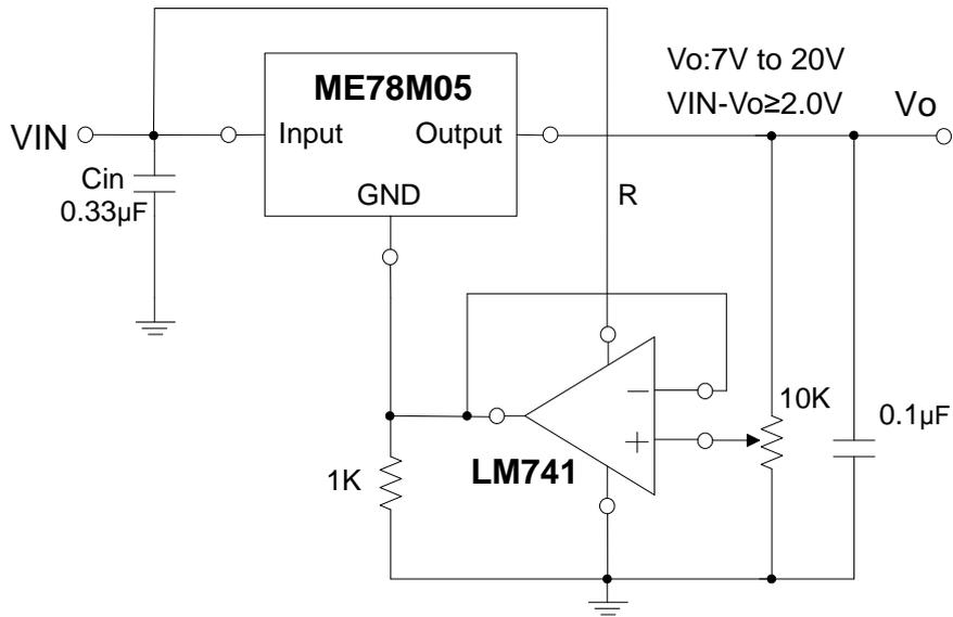
The addition of an operational amplifier allows adjustment to higher or intermediate values while retaining regulation characteristics. The minimum voltage obtainable with this arrangement is 2.0 V greater than the regulator voltage.
