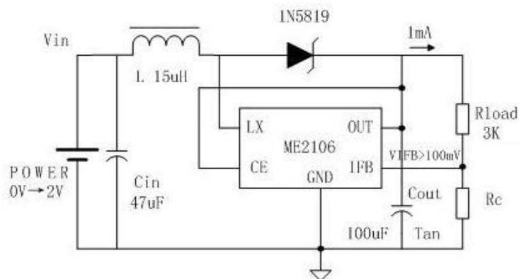
(3) Test holding voltage
