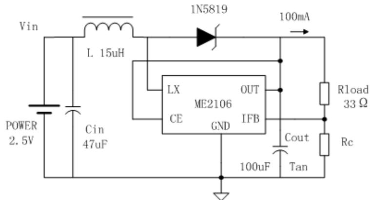
(2) Test startup voltage
